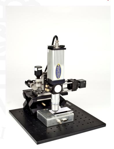
Camera used to get images of laser spots on the surface
